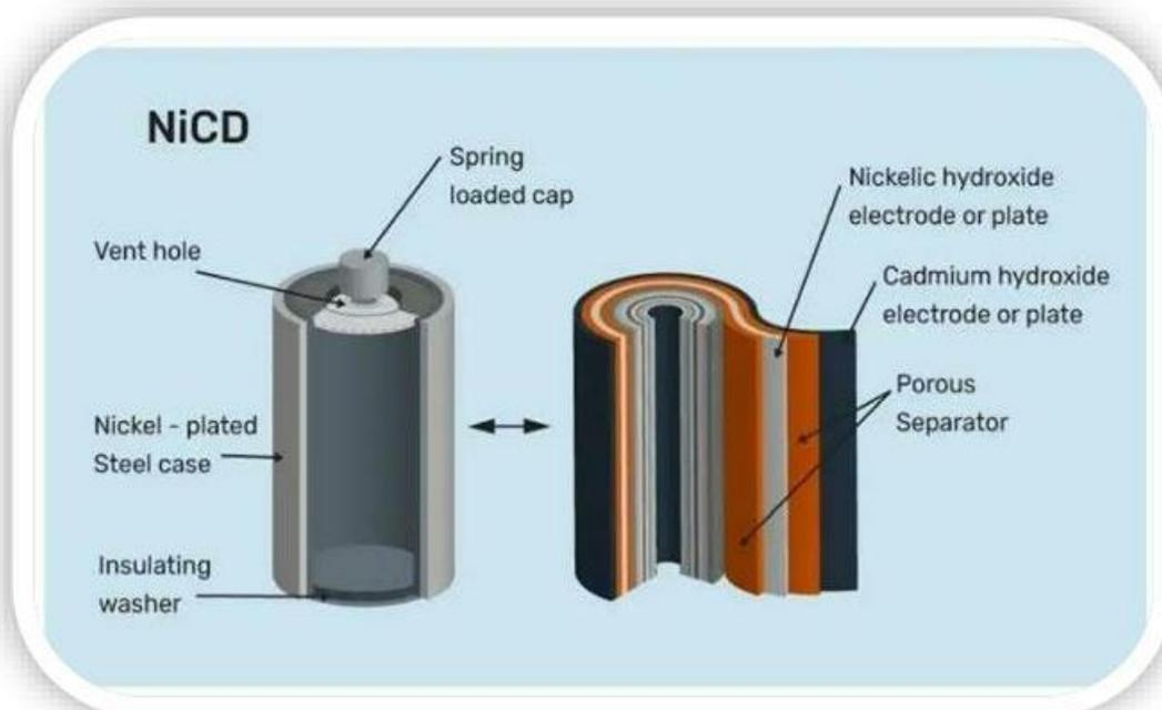
**Figure 02: La batterie Nickel-Cadmium (Ni-Cd) [6]** (la source: [What is a nickel-cadmium battery \(NiCd\)? - Independent Power Supply Systems Engineering \(powersystemscoach.com\)](http://www.powersystemscoach.com))
